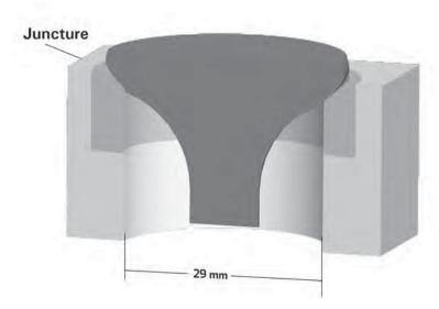
10. Replacement of intake and exhaust valve seats is allowed for the purpose of repair only. Valve Seats may not be moved from their original position. Welding is allowed to facilitate repair and installation of replacement seats. The original size and shape of the combustion chamber must be maintained. Installed seats may neither be proud or recessed of the combustion chamber surface.
